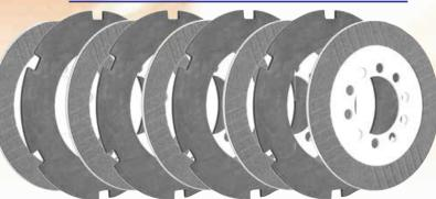
DESIGNED FOR USE ON 1941-EARLY 1984 BIG TWINS, THIS KIT INCLUDES FIVE KEVLAR FRICTION PLATES (6061 T6 ALUMINUM CORE) WITH MAXIMUM DEPTH GROOVE FOR EFFICIENT HEAT DISSIPATION, AND OIL CIRCULATION. ALSO INCLUDED ARE FOUR TEMPERED STEEL DRIVE PLATES. CLUTCH PACK HEIGHT IS PRE-SET FOR EASY INSTALLATION. (WET OR DRY). FRICTION PLATES REPLACE OEM 37930-68. STEEL PLATES REPLACE OEM 37975-41/81.
