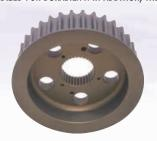
THESE PULLEYS WILL FIT 1993 to PRESENT BIG TWIN MODELS w/5 or 6-SPEED TRANSMISSIONS. TO RETRO-FIT THEM TO EARLY (1985-1993) 5-SPEED TRANSMISSIONS A LATE MODEL RACE/SPACER (#3217-0008) MUST BE USED AS WELL AS A NEW SEAL(#12067A). ALSO, WE RECOMMEND INSTALLING A QUAD SEAL ON THE HIGH GEAR.
