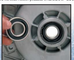
SIMPLY REMOVE THE OEM RACE FROM THE TRANSMISSION MAINSHAFT BY USING TOOL #34902-84.
