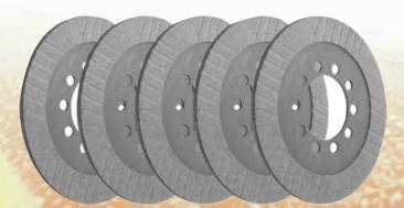
THIS CLUTCH PACK KIT IS FOR USE ON 1941-1984 BIG TWINS. IT INCLUDES FIVE KEVLAR FRICTION PLATES WITH TEMPERED STEEL CORES. MAXIMUM GROOVE PATTERN FOR EXCELLENT HEAT DISSIPATION & OIL CIRCULATION. RUN THESE WET OR DRY.
