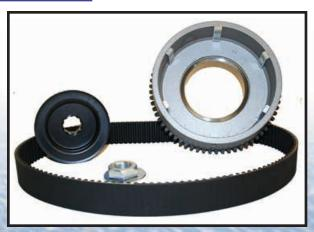
1-1/2" BELT DRIVES ARE DESIGNED FOR USE W/STOCK DISPLACEMENT MOTORS. PRIMARY BELT STRENGTH IS PROPORTIONAL TO BELT WIDTH.
